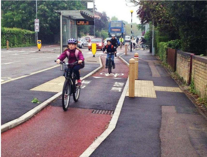
Fig 3. Segregated, continuous cycle track running behind the bus stop
